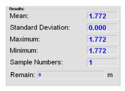
**Note:** statistics shown on the "Results" pane are compiled by the PCIS\_DGK software using raw diameter data collected from the gauge and may not correspond to statistics computed by the gauge.
